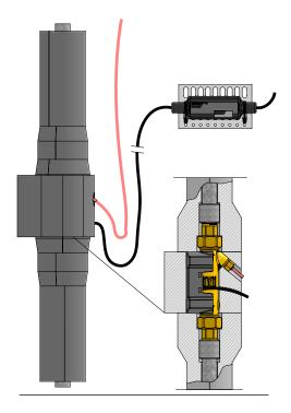
ULTRAFLOW® 44 tolerates periodical submersion. This applies to the meter housing as well as the electronics (PCB) of ULTRAFLOW® 44. If ULTRAFLOW® 44 is flooded, the connected MULTICAL® must not be flooded. Furthermore, temperature sensors must also not be flooded and therefore must be mounted elsewhere in the installation.
