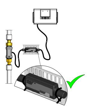
Must NOT be mounted on flow sensor or on pipes
