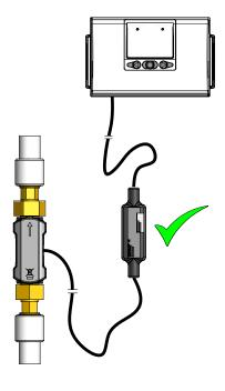
Horizontally mounted with cable strips in humid environments
